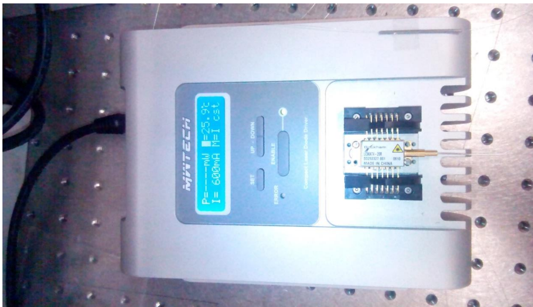
Figure 6: Picture of the laser diode used as source to achieve optical pumping of the system
