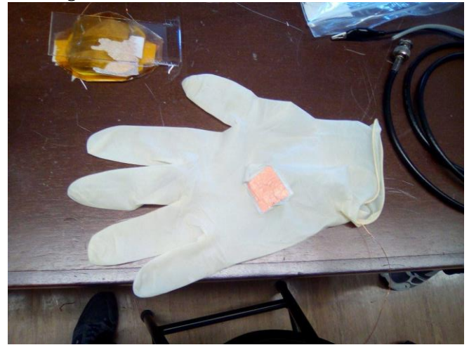
Fig.10 – Image depicting the electrode outside the glove, connected to the skin inside the glove
